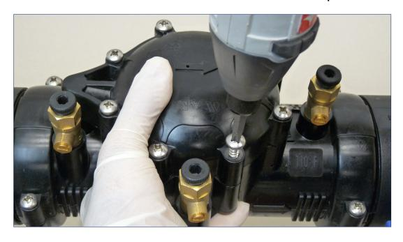
The RP-501 Cover is spring loaded and sealed by 8 stainless steel screws. The Relief Diaphragm is spring loaded and secured in the cover. \*\* Hold Cover firmly while removing the Screws..
