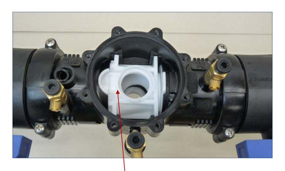
Remove the <u>Retainer</u> by pulling straight up to get access to the #1 and #2 Check Modules.
