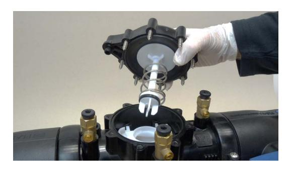
After releasing the screws, remove the cover with secured relief diaphragm.
